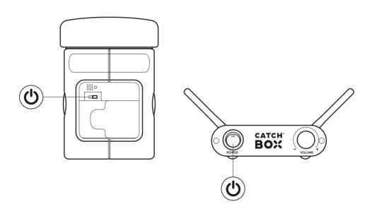
Place the transmitter into the cover, making sure to align the magnetic locking mechanism so it is secure. Use the visual marks for guidance.
